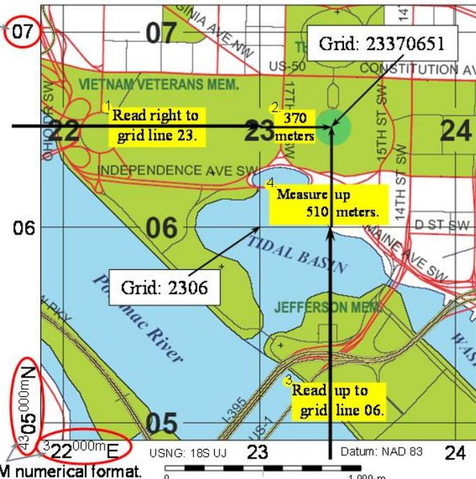
Ignore the small UTM superscript numbers that are provided for reference purposes. UTM numerical values are best suited for determining direction and distance as in surveying. USNG alpha-numeric values are best suited for position referencing because they can be given as only grid coordinates in a local area and with only the required precision for a particular task.
