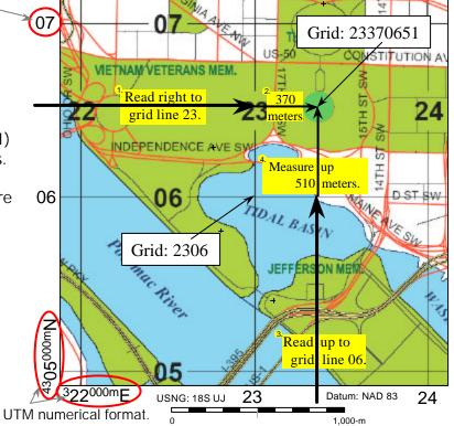
Ignore the small UTM superscript numbers that are provided for reference purposes. UTM numerical values are best suited for determining direction and distance as in surveying. USNG alpha-numeric values are best suited for position referencing because they can be given as only grid coordinates in a local area and with only the required precision for a particular task.
